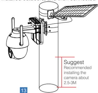
Suggest Recommended installing the camera about 2.5-3M
